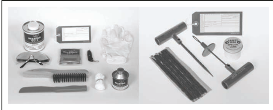
Figure 6-10. Tire patch materials and tire plug kit
