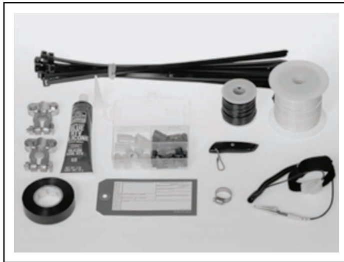
Figure 6-9. Electrical repair materials
